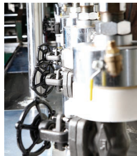
Gate/Globe valve testing station
