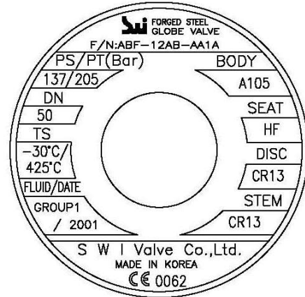
Globe valve / Bellows globe valve
